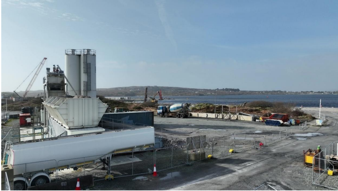
Figure 2-28: Photograph of the mobile Concrete Batching Plant and water storage tank.
